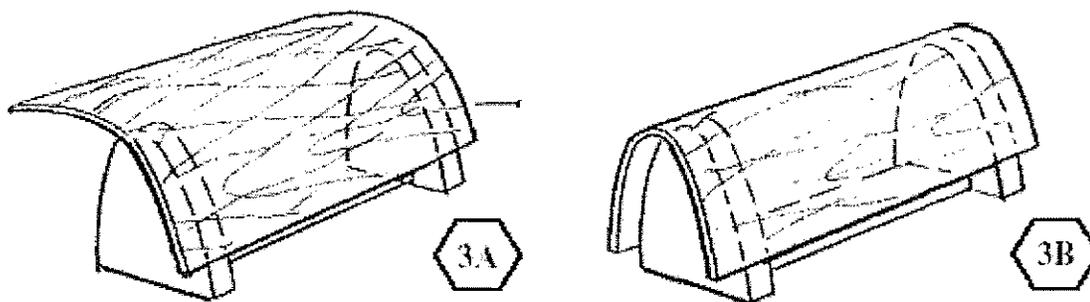
After the felt has been applied to the form a squaring block must be screwed to the form. It is on what will be the top part of the leading edge of the wing and is 2 1/2 inches back from the leading edge along the cord and is parallel with the leading edge. Figure 4A shows why this block is necessary. The squaring block is made from a piece of pine and can be attached with two 1 1/2 inch #8 drywall screws. The squaring block is 2 1/2 inches aft of the leading edge on the top of the wing
