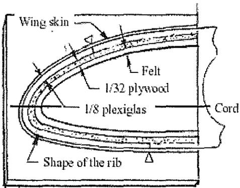
Cut a board 4.5" x 3.5" to place between the two airfoil shapes. Make sure cord lines are on the same plane. Screw and glue together. Use white glue and drywall screws. See figure 2A. This completes
