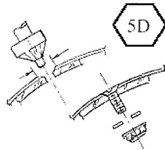
Step 6. With lens held in place with a couple of temporary screws it is time to locate the hinge that will be the main support for the light and give the light the ability to be adjusted to different angles. The hinge
