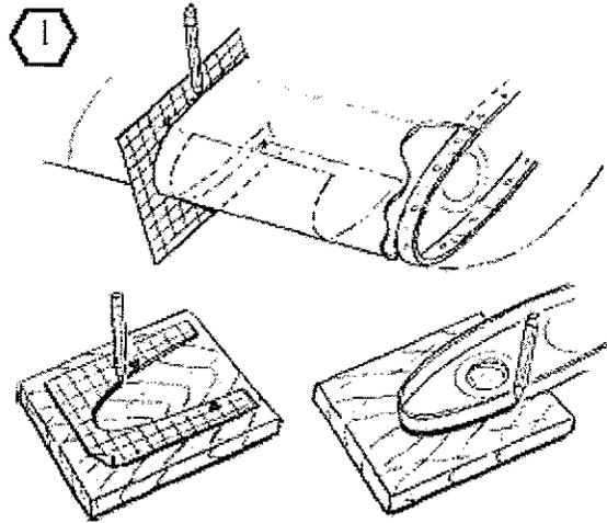
**Step 2.** After forming two pieces the shape of the rib, material must now be removed to allow for the thickness of the plexiglas, plywood covering and felt which will cover the form to keep from scratching the Plexiglas while forming. Cut shape on band saw to the line marked felt. Leave the line and sand to the line on disk sander.
