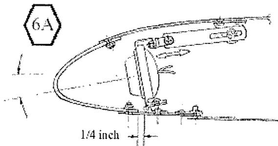
should be located 1/4 inch aft of the bottom rear of the lens. Center hinge behind the lens and drill with #40 drill and cleco through holes provided. Be sure to use the hinge half marked bottom. Dimple the skin and countersink the
