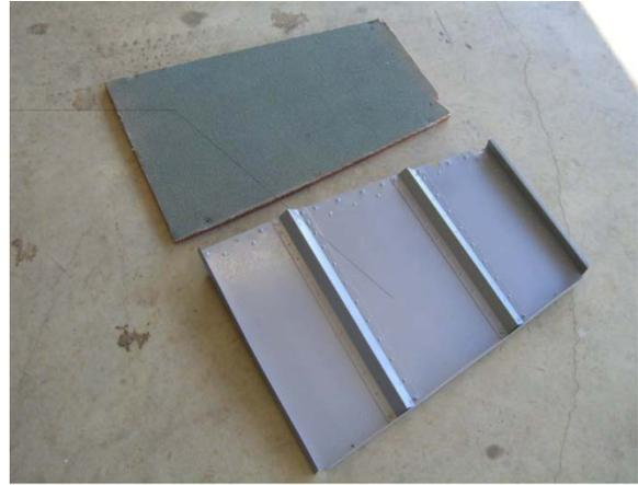
New baggage compartment floor panels (and rear panel) were made from .025 sheet stock. Original panel on left is a composite material with glued carpet. Weight difference between the two parts is negligible.
