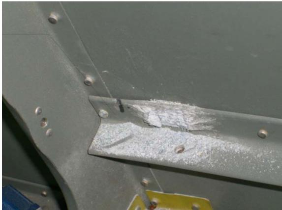
Severe exfoliation corrosion of left side fuselage intermediate longeron. This longeron supported left side baggage compartment floor panel.
