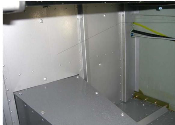
New baggage compartment aft panel, floor panel and tunnel installed. Tunnel was made using original parts as templates. Everything was finished in paint and can be easily inspected.
