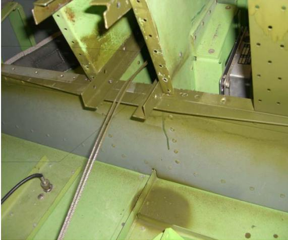
Aft looking forward- four  $\frac{3}{4}$  x  $\frac{3}{4}$  x  $\frac{1}{16}$  inch angles in tunnel 505 replaced due to corrosion. Forward end of baggage compartment tunnel is attached to these angles. Corrosion removed to ~ 20% depth in upper carry through spar cap at location of tunnel interface. A double tapered angle doubler was riveted to the aft side to maintain structural integrity.
