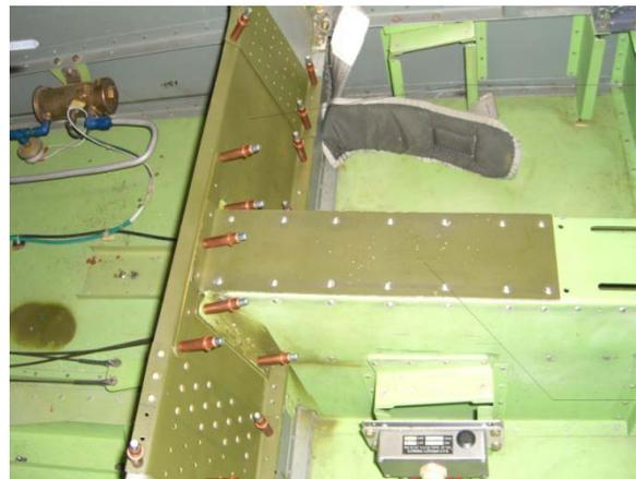
Bulkhead 598 splice- Material with the dark colored primer is new. Each end has .040 inch doubler plates requiring ~23 rivets on each side of the splice. Top of tunnel 505 between seats was replaced due to a crack found in aft flange.
