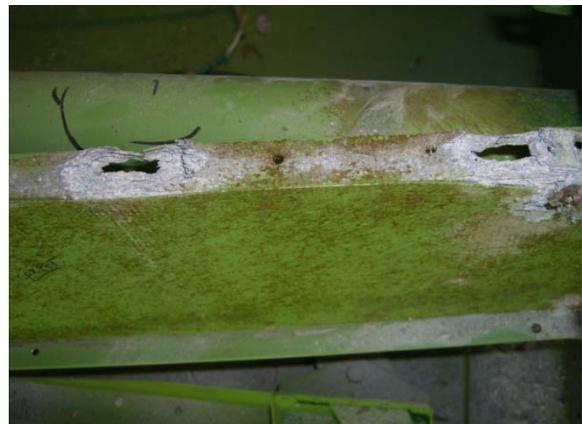
Baggage compartment tunnel side panel damage at steel anchor nut screw locations where tunnel top piece attached. Carpet has been removed in this picture.
