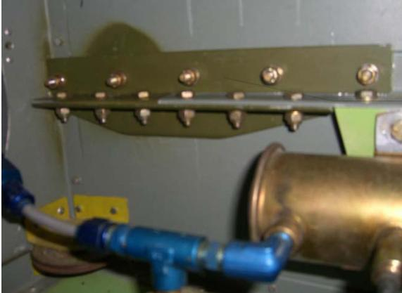
Removed ~ 3 inches of left hand side intermediate longeron 580-5. Spliced new angle material using 1x1x1/8 double tapered angle on the bottom and 1x1/8 bar stock on upper leg. Six AN3 bolts attach the lower section and AN525 bolts attach the upper section. This unfortunately leaves protruding round heads on the fuselage exterior skin which is otherwise all flush riveted.
